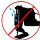
**NEVER** apply direct water pressure to the electronics
